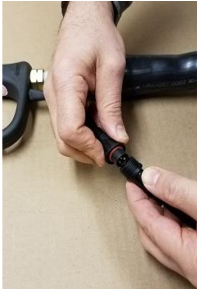
Connect 3-Pin electrical connection between Hose and Autoshot
