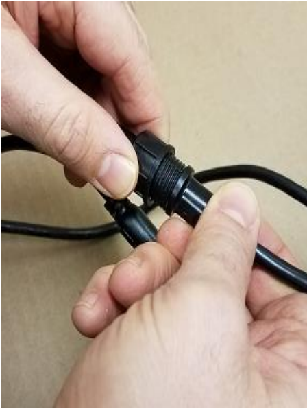
Connect 5-Pin electrical connection between Pump and Hose
